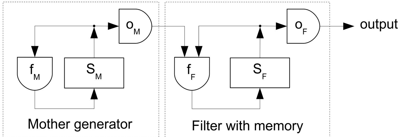
The combined generator can be regarded as an automaton with state space  $S_M \times S_F$  without input.
